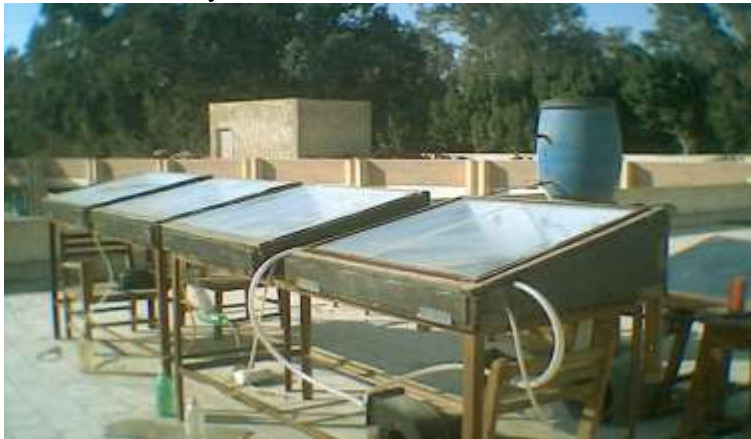
Fig. (2) Four solar still units.
