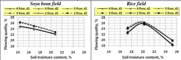
Fig. (9): Degree of soil plowing quality by using different shapes of chisel plow under different soil moisture contents and plowing depths.
