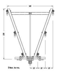
Fig. (2): Modified  $\Delta$ -shape chisel plow (4 rows).
