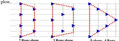
Figure (1): Arrangements of the 7 tines of modified  $\Delta$ -shape chisel plow (4 rows) compared with 2 and 3 rows shapes of chisel plow.
