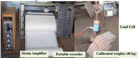
Fig. (5): Calibrating measuring draft force system.
