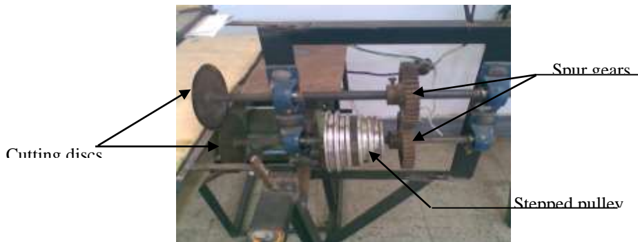
Fig. 3: Trimming unit and transmission mechanism.
