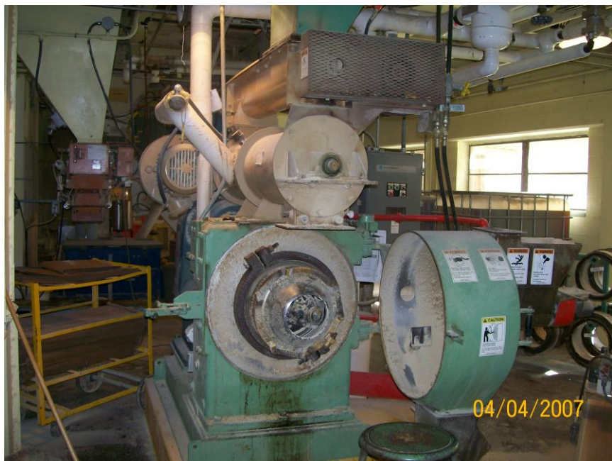
Fig.(4): California pellet mill ring die (CPM)
