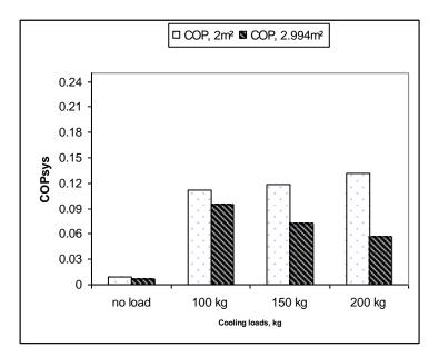
Fig.3: The COP<sub>sys</sub> values with different cooling loads under fluid flow rate of 7.5 l/min and two solar collector areas.
