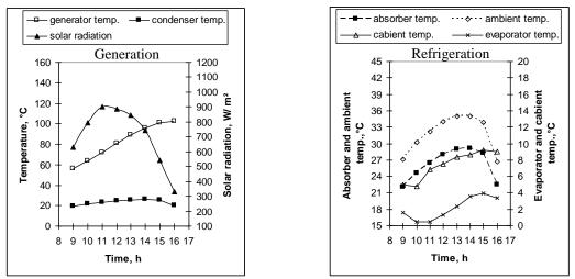
Fig. 9: Observations on the solar refrigeration cycle during generation and refrigeration for fluid flow rate of 2 l/min under condition of 200 kg potato load with 2  $m^2$  solar collector areas.
