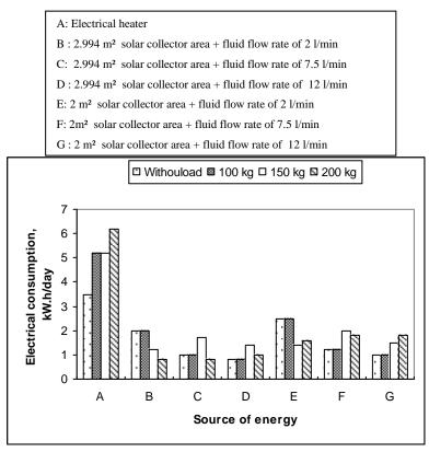
Fig. 6: The electrical consumption and source of energy under different cooling load conditions.
