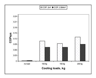
Fig.2: The  $\text{COP}_{\text{sys}}$  values with different cooling loads under fluid flow rate of 2 l/min and two solar collector areas.
