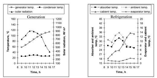
Fig. 8: Observations on the solar refrigeration cycle during generation and refrigeration for fluid flow rate of 2 l/min under condition of withouload with  $2 \text{ m}^2$  solar collector areas.
