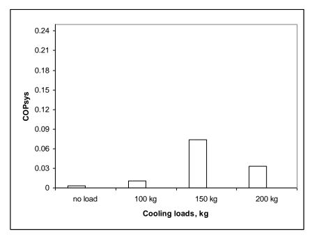
Fig. 5: The COP<sub>sys</sub> values with different cooling loads under electrical heater
