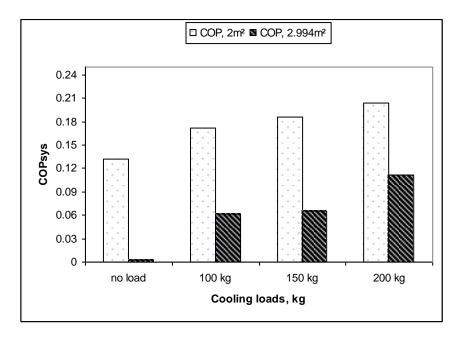
Fig. 4: The COP<sub>sys</sub> values with different cooling loads under fluid flow rate of 12 l/min and two solar collector areas.
