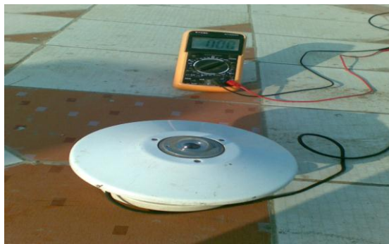
Fig. (3): The pyranometer device and digital voltammeter used to measure the solar radiation flux incident.
