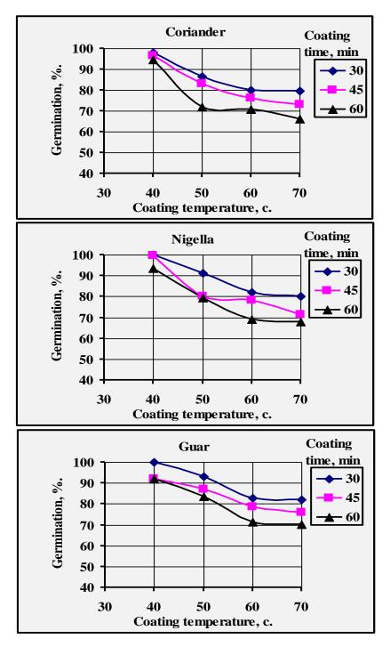
Fig. 3: Effect of coating temperature and time on germination of coriander, nigella and guar seeds.
