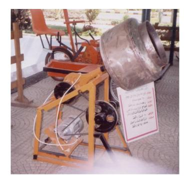
Fig. 1: Sketch and photograph of the coating machine (Yehia, 2008).
