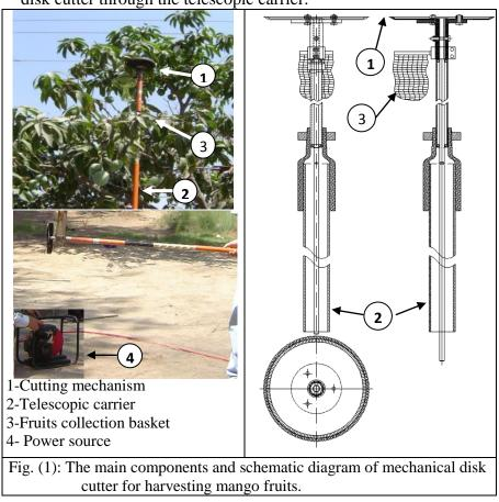
• The cutter shaft was used to transmit the power from clutch to the disk cutter through the telescopic carrier.
