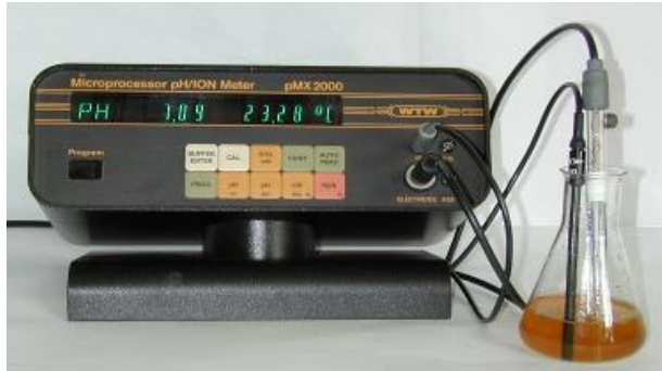
Fig.4. Instrument for measuring the pH value of Straw
