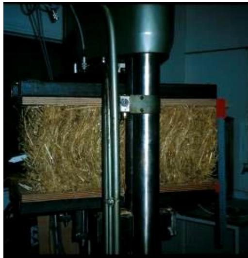
Fig.6. Straw bale in compression test
