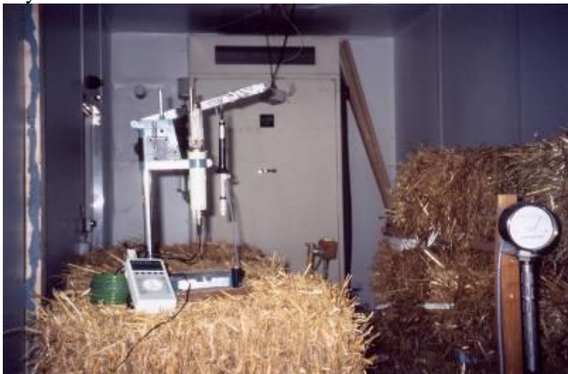
Fig.5. Bales inside the climate chamber under compensation test condition
