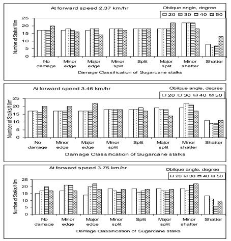
Fig. (8) Effect of forward speed on damage classification of sugarcane stalks **4. Collecting efficiency**:
