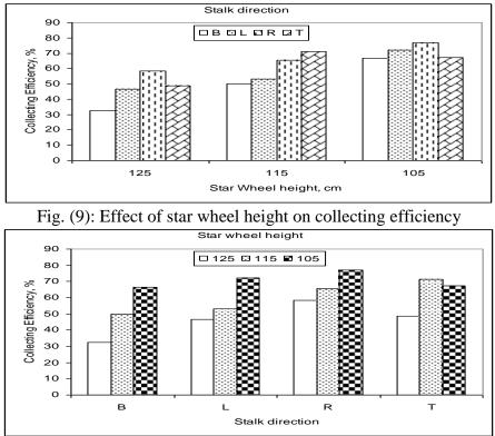
Fig. (10): Effect of stalk direction on collecting efficiency
