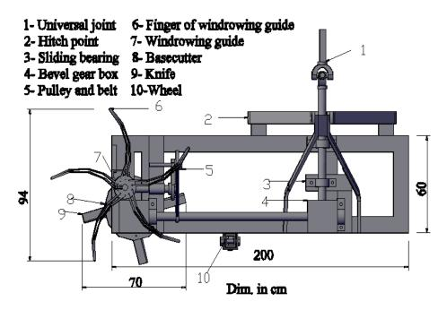
Fig. (2): Plane view of the developed sugarcane harvester
