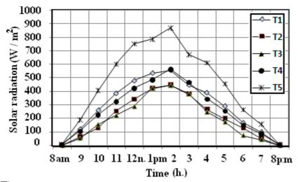
Fig. (2): Diurnal variation\* in transmission of solar energy in different poly-greenhouse models for the month of April, 2010.
