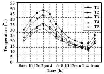
Fig. (4): Diurnal variation\* in air temperature outside and inside the poly-greenhouse models during the day-time of April, 2010.
