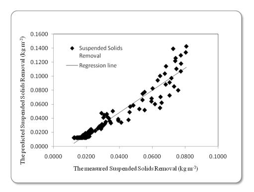
Fig. (4) The predicted and the measured suspended solids removal from the system (RAS)
