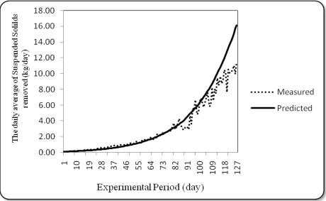
Fig. (5) The daily average of suspended solids removed by drum filter (kg/day)
