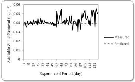
Fig. (2) The predicted and the measured settleable solids removed from the system (RAS).
