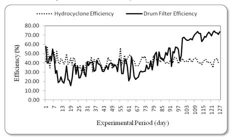
Fig. (6) The efficiency of the removal settleable and suspended solids (%)
