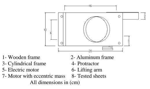
Fig. (3): Elevation side view and plan of the apparatus used to measure the static coefficient of friction.
