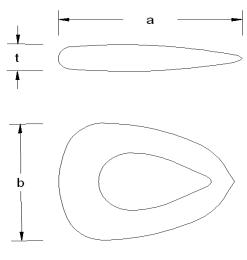
a = Length of the seed b = Width of the seed t = Thickness of the seed
