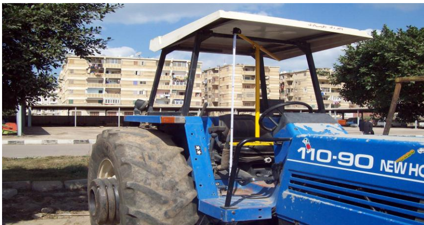
Fig.3. Designed device stands at SRP during measurements (Cabin without sound glass guard).
