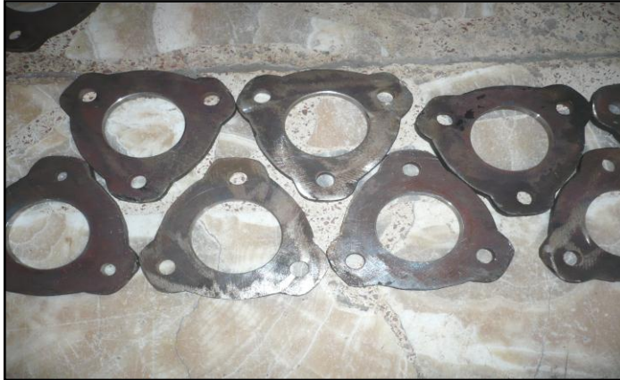
Fig. 5. Photograph of barrel rings with circular spacers
