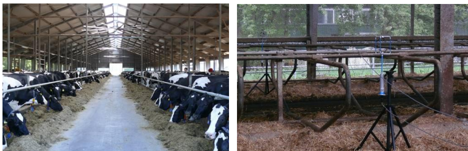
Fig. 1: Internal view of the barn showing the ceiling fans (left) and used ultrasonic anemometer (right).
