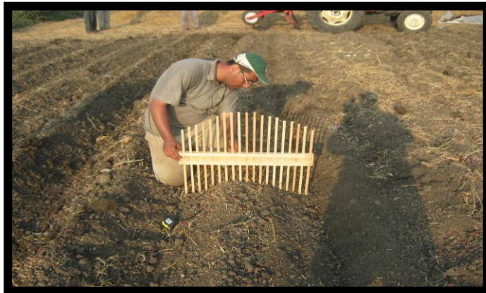
Fig. (3-4) Measuring soil profile.
