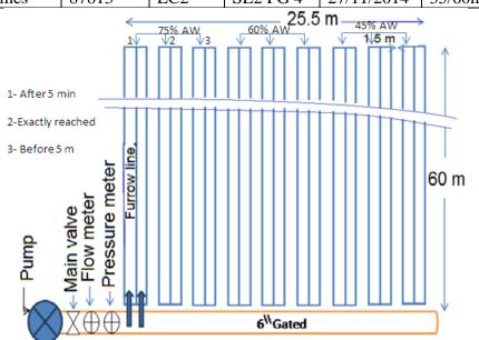
Fig.1. Layout of experimental replicate
