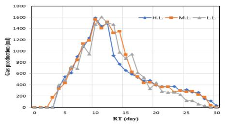
Figure (8): Gas production for laboratory-scale reactors
