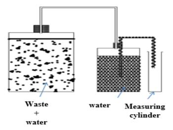
Figure (1): Laboratory- scale reactors set-up
