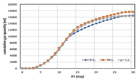
Figure (9): Cumulative gas quantity for laboratory-scale reactors
